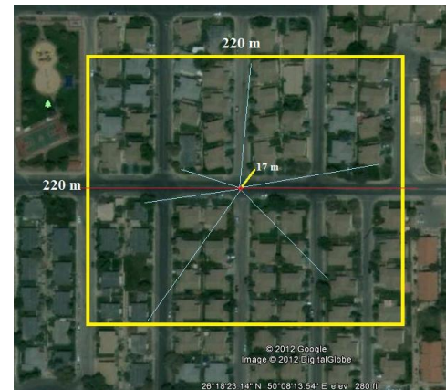
Figure 5. 64-buildings in Al-Dhahran with Single BS located at the center of the scenario
