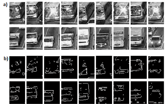
Fig. 7. Images classified incorrectly in level 2, features NP+W+F+BW, classifier SVM RBF : a) Vehicle images b) Vehicle edge
