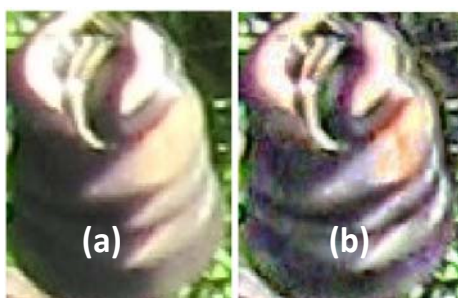
Fig. 3. Example of application of contrast adaptive equalization: (a) Original image (b) Image with contrast equalized.
