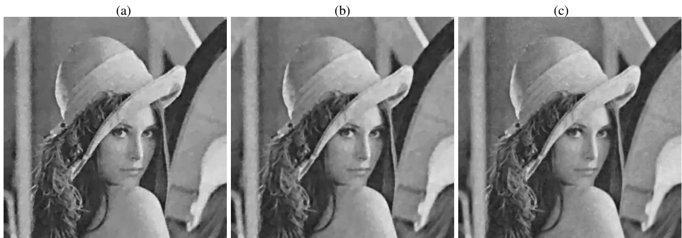
Fig. 2: Lena: Restored images by (a) \mathcal{M}_1 , (b) \mathcal{M}_2 , and (c) \mathcal{M}_3 . The restored images show PSNRs of 31.1, 31.1, and 31.3 respectively for \mathcal{M}_1 , \mathcal{M}_2 , and \mathcal{M}_3 .
