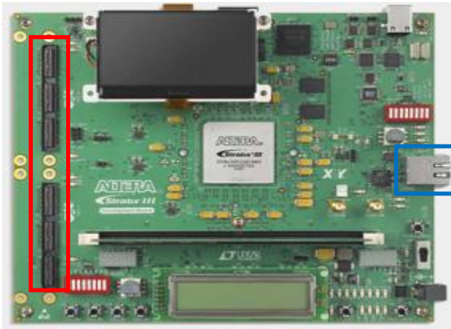
Figure 2. The Virtual Bus Interface System Implementation with Interface Connections on the Altera Stratix III Development Board
