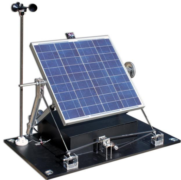
Figure 6: Finished Solar Tracker System
