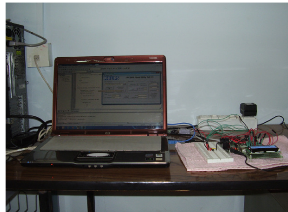
Fig1: The mini ARM kit connected to the laptop and program uploading window
