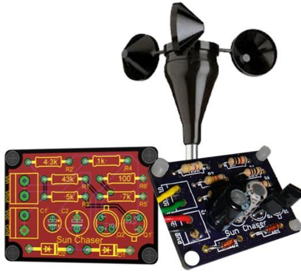
Figure 2: Anemometer, PCB, and Completed Analog-to-TTL Circuit Board
