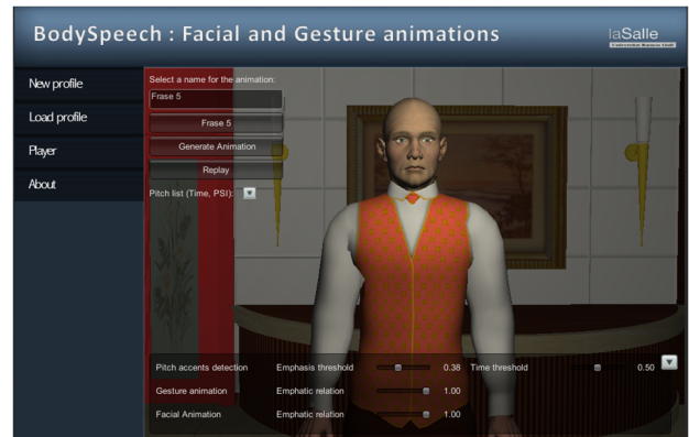
Fig. 9: Synthesis screen. On the upper-left corner, there are the buttons to select an audio and generate the animations. At the bottom, there are the configurable pitch accent detection parameters, and sliders for adjusting gestural or facial animation emphasis.
