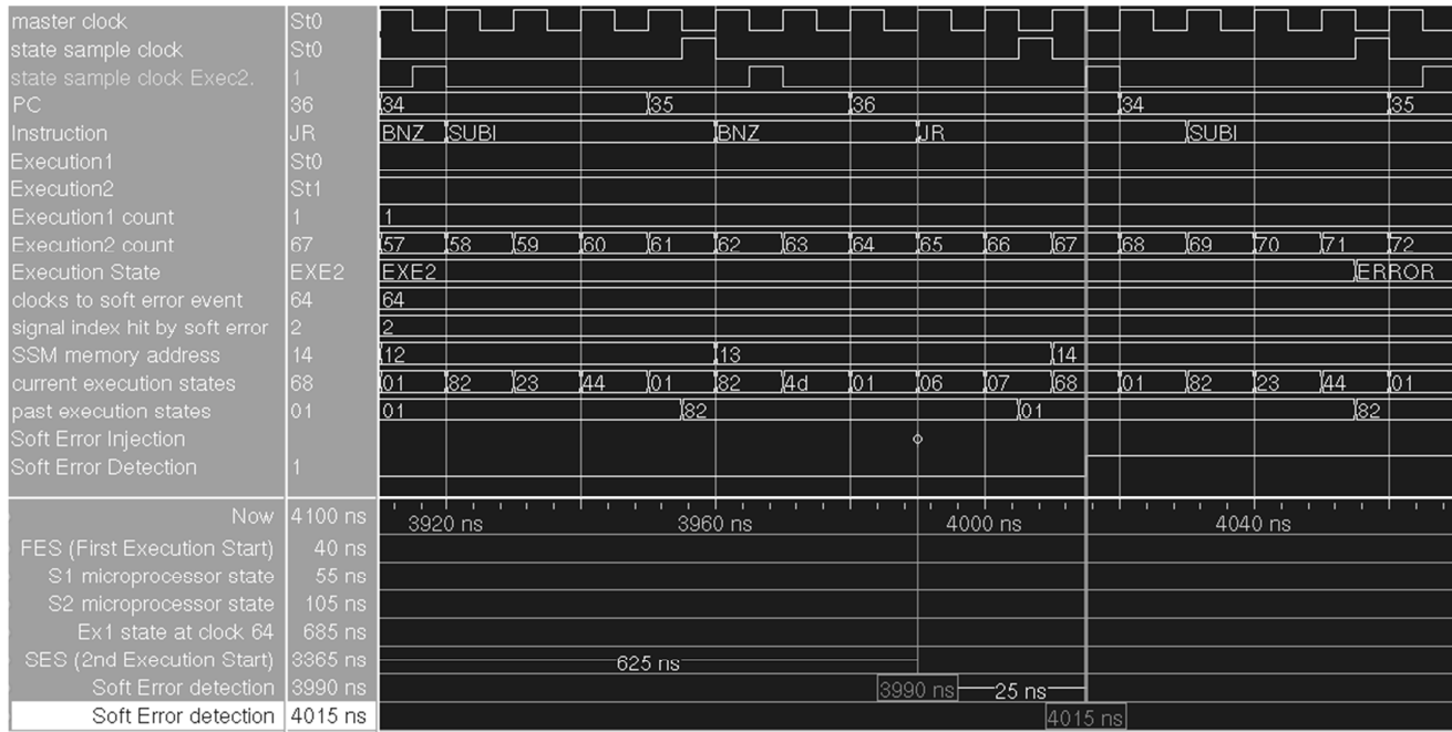
Fig. 8. Second execution: The soft error occurs at time 3990 ns and it is detected at 4015 ns.
