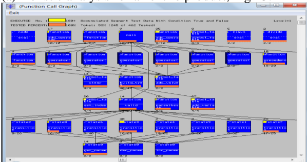
Fig. 13 Holistic MC/DC (Modified Condition/Decision Coverage) test coverage analysis
