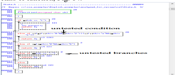
Fig. 14 An application example of detailed test coverage analysis of a module
