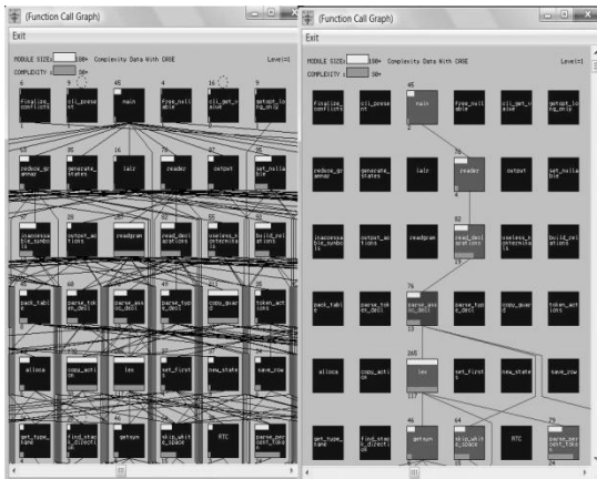
Fig 2 An automatically generated call graph shown with the cyclomatic complexity (the number of decision statements such as 'if', 'for', 'while', 'do', 'switch') measurement result and a module highlighted with the all related modules calling and called by it
