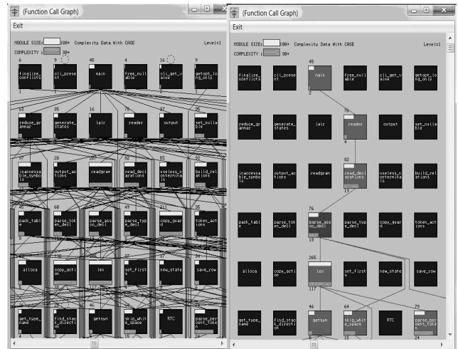
Fig. 5 A call graph of a entire software product designed (on the left side) and a module with its all related modules traced/highlighted
