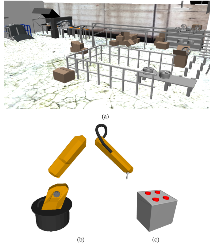
Fig. 1: (a) The 3D factory hall includes the structure and accessories. (b) The single parts of the industrial robot. (c) A simple console with buttons, meant to rotate the segments of the robot.
