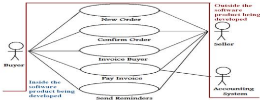
Fig. 21 Actors of a Use Case diagram are outside the software product under development.
