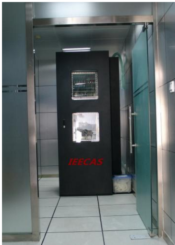
Fig.5 Prototype of spray evaporative cooling HPC
