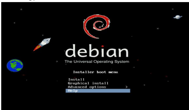
Figure 3. Step1 - boot the server with a genuine Debian CD-ROM and select “Help”
