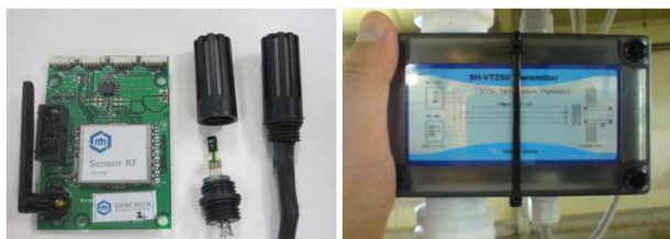
Figure 11. Environmental Sensor and CO2 Sensor
