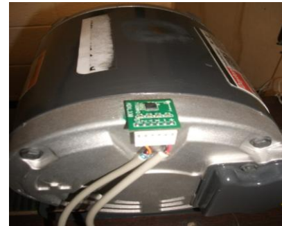
Fig. 8 A accelerometer mounted on the motor housing
