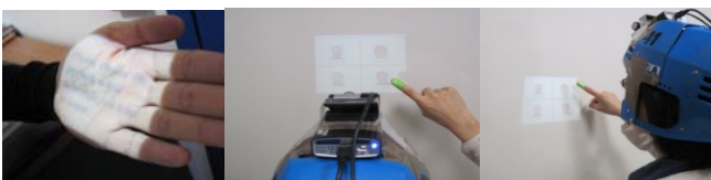
Figure 5 Environment Independent Interface (EII) a) information projected on the palm b) Camera and picoprojector configuration c) information projected on the wall
