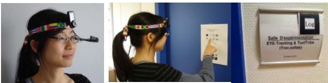
Figure.4 Environment Dependent Interface (EDI) a) Camera and goggle based screen configuration b) c) in-environment markers
