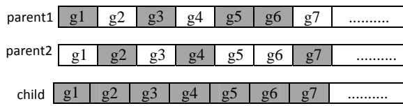
Fig. 5: Crossover Operator, selecting gene1 from parent1 and transmitting this gene to the child with its related genes. This is true for gene2 from parent2.
