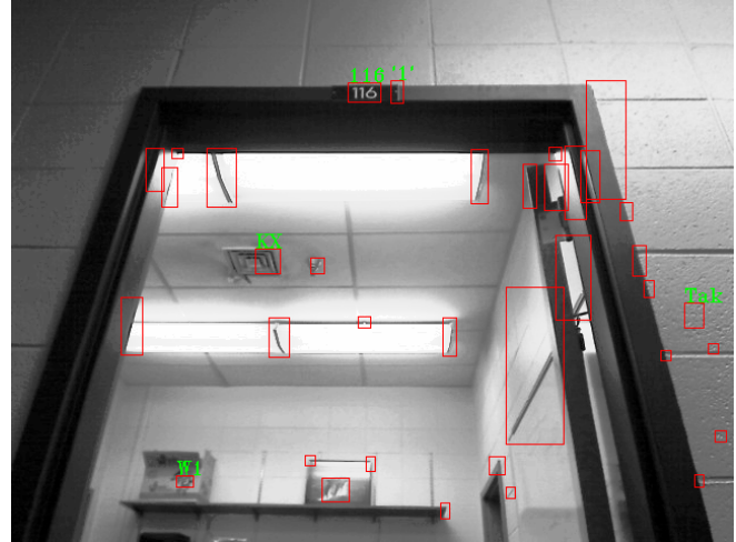
Fig. 3: Results of text detection, as indicated by the red boxed regions, and the results when passing that area of the higher resolution image to the OCR engine.
