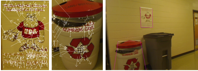
Fig. 1: (Left, Center) SIFT Features on two sample objects. The arrows indicate the keypoint's orientation and scale at which it was found. (Right) Example of object recognition using the two sample object models, with the top of the object indicated with a white line.
