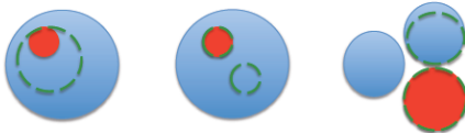
Figure 1. Three cases of parent filler (red and blue), selected child filler (red), correct child filler (dotted green)
