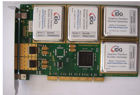
Fig. 1: Quantis RNG Card for PCI Bus, showing four independent quantum generator devices.
