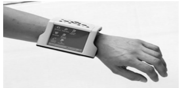
Fig 3.5.1 Novel TMS320 DSP based Multipara System
