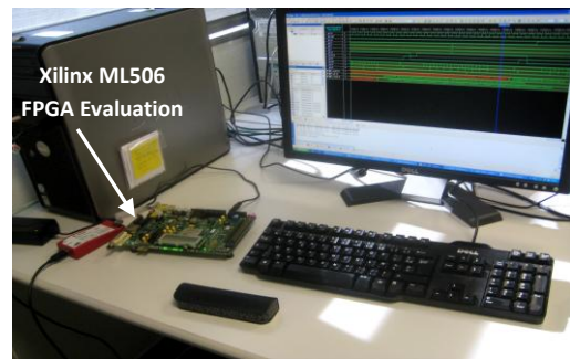
Figure 5, Hardware in Loop
