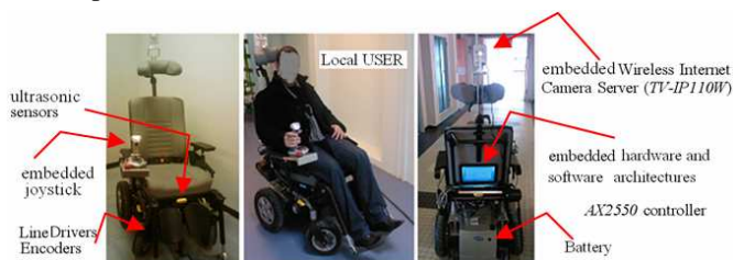
Figure 1. LIASD-WheelChair structure
