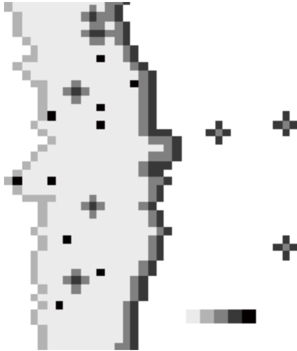
Fig. 1: Schematic representation of the states in the CA model for passive layer. The grey scale codes are as follows. Metal (M) bulk sites (on the left hand side) and solution (S) bulk sites (on the right) are blank as no storage is reserved for them in the program. The bar indicates the grey code for inactive oxide, active metal, active oxide, active solvent and active walker from left to right respectively.
