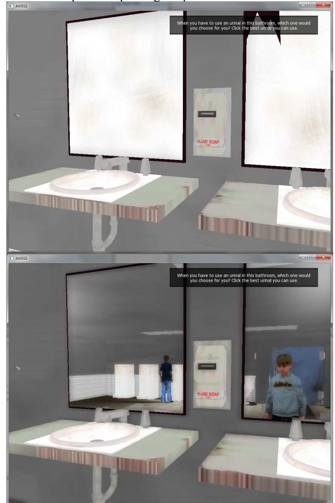
Figure 1-2: Comparisons of Local and Global AViSSS. The top figure shows the restroom with local lighting and the bottom shows the restroom with global lighting. Notice the accurate rendering of the mirrors and shadows in the global version of AViSSS.
